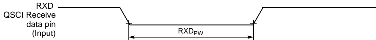
Figure 10-12 RXD Pulse Width
